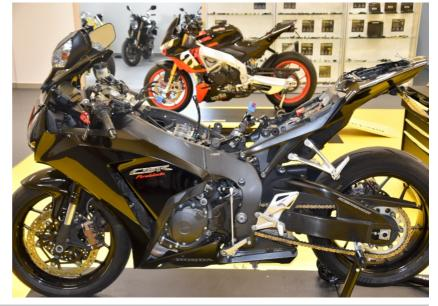
Locate the stock electronic steering damper and unplug the connector.
