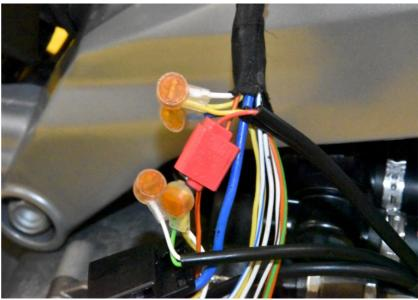
Splice the SH Black wire to the Blue wire of the unused additional connector. Use a red wire tap connector.
