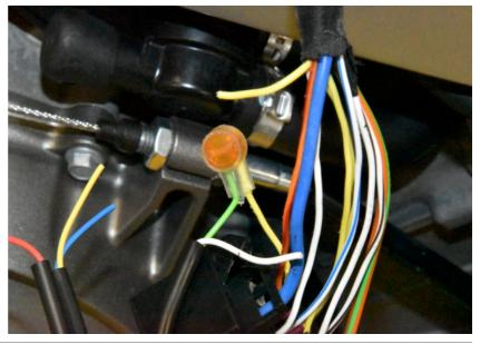
Connect the SH Blue wire to the Yellow wire end, which is at the wiring harness side. Use a yellow butt connector.
