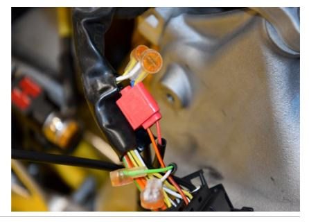
Splice the SH Black wire to the Blue wire of the fuel pump connector. Use a red wire tap connector.
