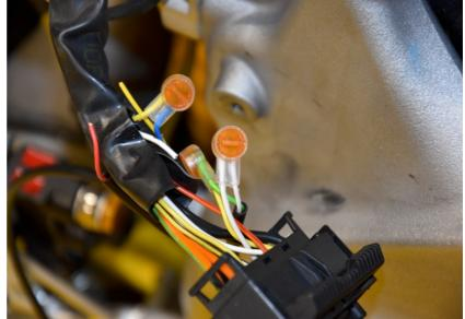
Connect the SH Yellow wire to the White wire end, which is at the wiring harness side. Use a yellow butt connector.
