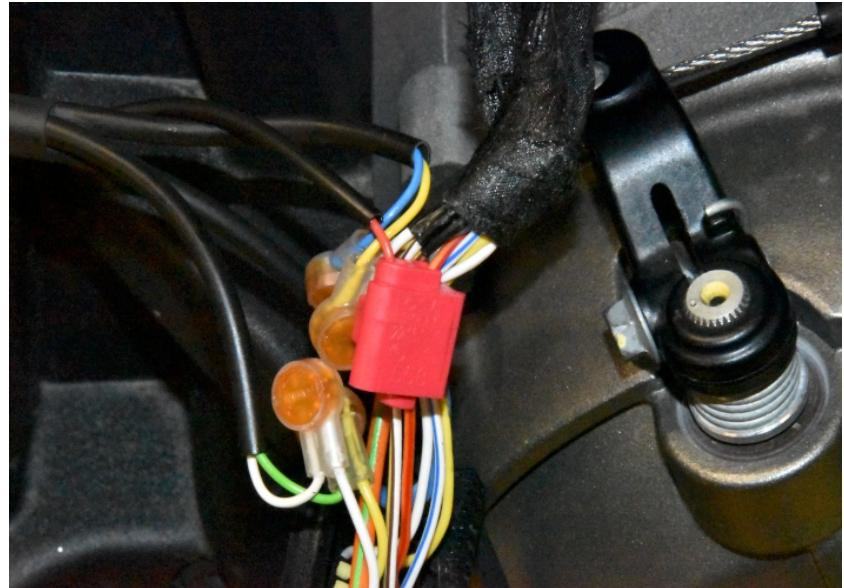
Splice the SH Black wire to the Black wire of the fuel pump connector. Use a red wire tap connector.
