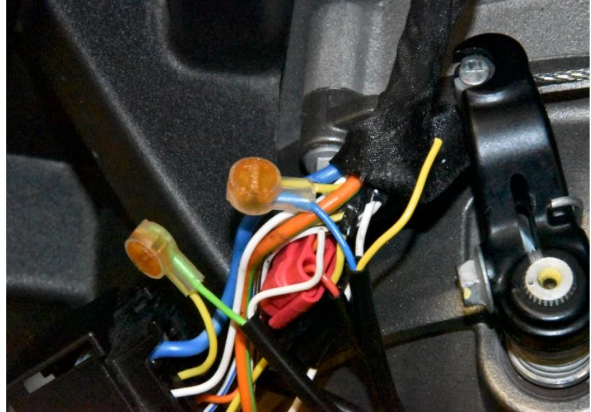
Cut the White wire about 2,5cm (1") of the connector. (Pin #11)
