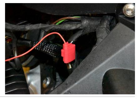
Splice the SH Black wire to the Brown wire of the dashboard connector. Use a red wire tap connector.
