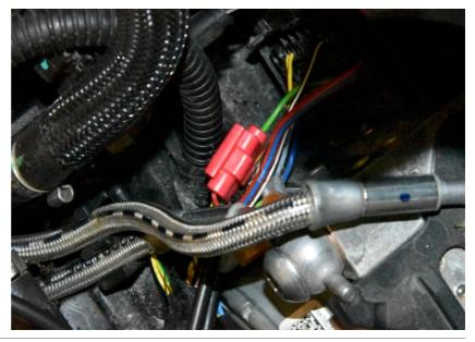
Splice the SH Black wire to the Brown wire of the additional connector. Use a red wire tap connector.
