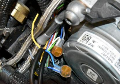
Connect the SH Yellow wire to the Grey wire end, which is at the wiring harness side. Use a yellow butt connector.
