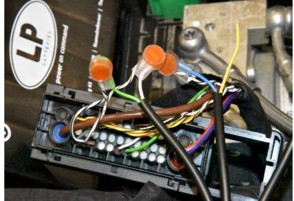
Connect the SH Yellow wire to the White/Brown wire end, which is at the wiring harness side. Use a yellow butt connector.
