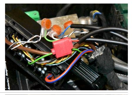
Splice the SH Black wire to the Brown wire of the diagnostic connector. Use a red wire tap connector.
