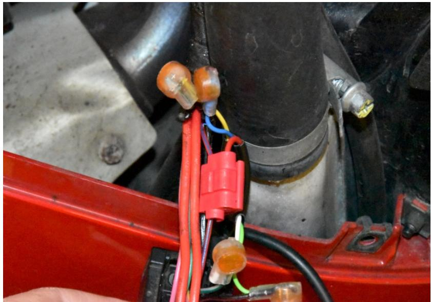
Splice the SH Black wire to the Grey wire of the ECU connector. Use a red wire tap connector.
