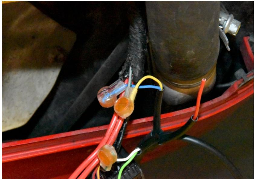
Splice the SH Red wire to the Red/Blue wire of the ABS connector. Use a red wire tap connector.
