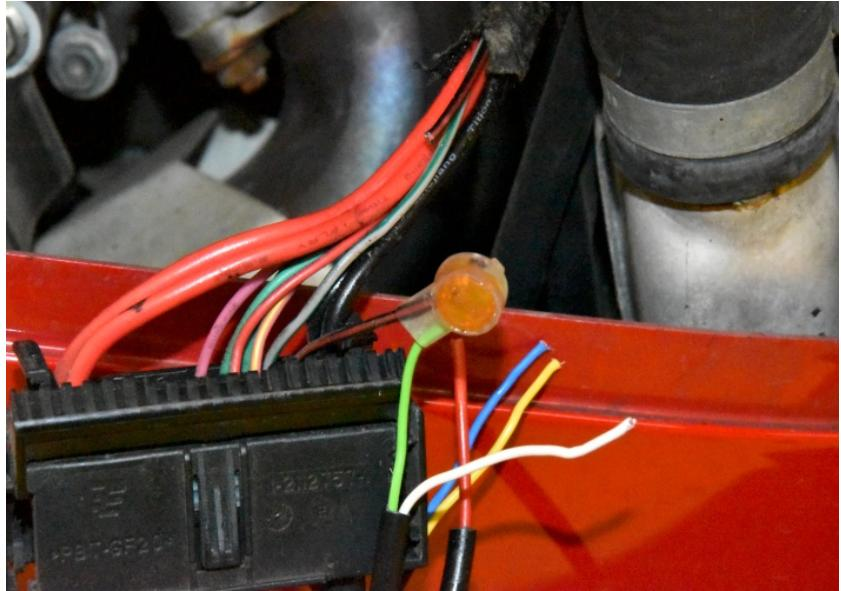
Connect the SH Blue wire to the Black/Brown wire end, which is at the wiring harness side. Use a yellow butt connector.
