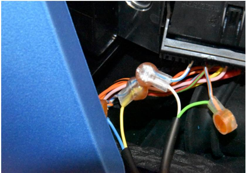
Splice the SH Red wire to the Red/Green wire of the ABS connector. Use a red wire tap connector.
