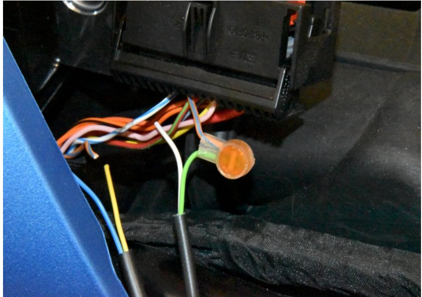
Connect the SH Blue wire to the Orange/Blue wire end, which is at the wiring harness side. Use a yellow butt connector.
