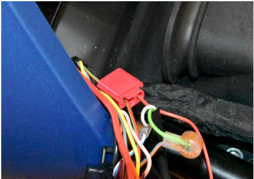
Splice the SH Black wire to the Black wire of the auxiliary connector. Use a red wire tap connector.
