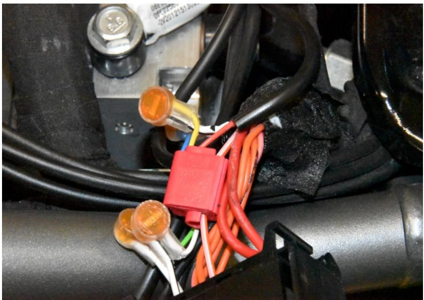
Splice the SH Black wire to the Black wire of the diagnostic connector. Use a red wire tap connector.
