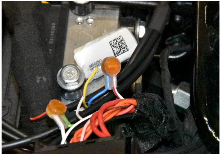
Cut the White/Black wire about 2,5cm (1") of the connector. (Pin #11)
