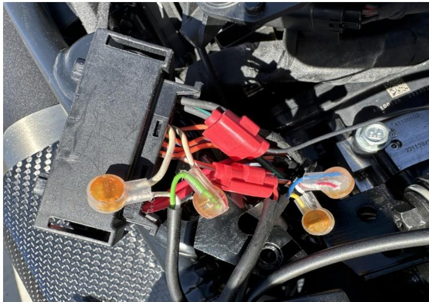
Splice the SH Black wire to the Black/Green wire of the ABS connector. Use a red wire tap connector.
