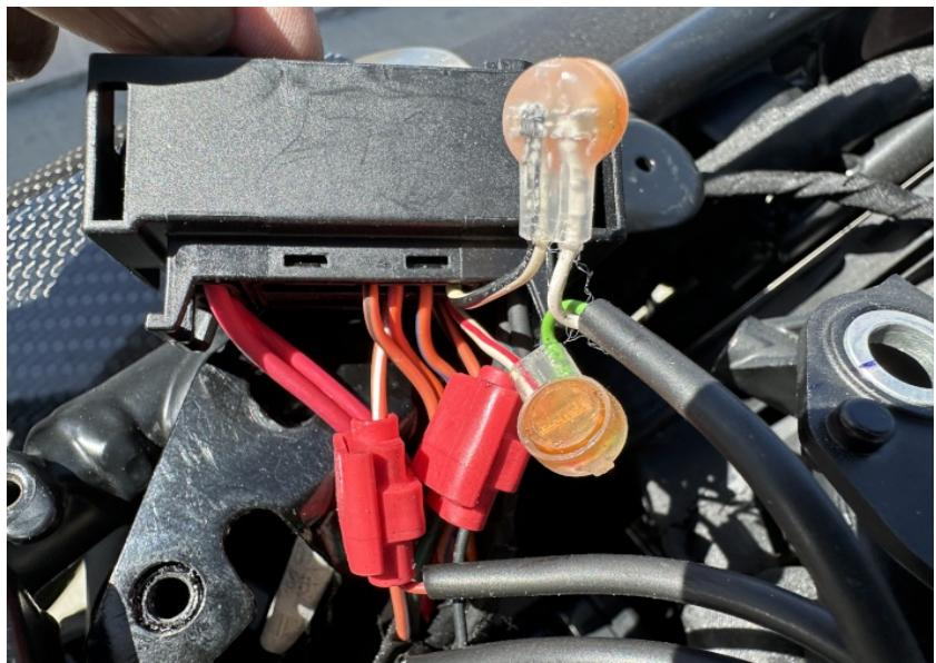
Connect the SH Blue wire to the White/Red wire end, which is at the wiring harness side. Use a yellow butt connector.
