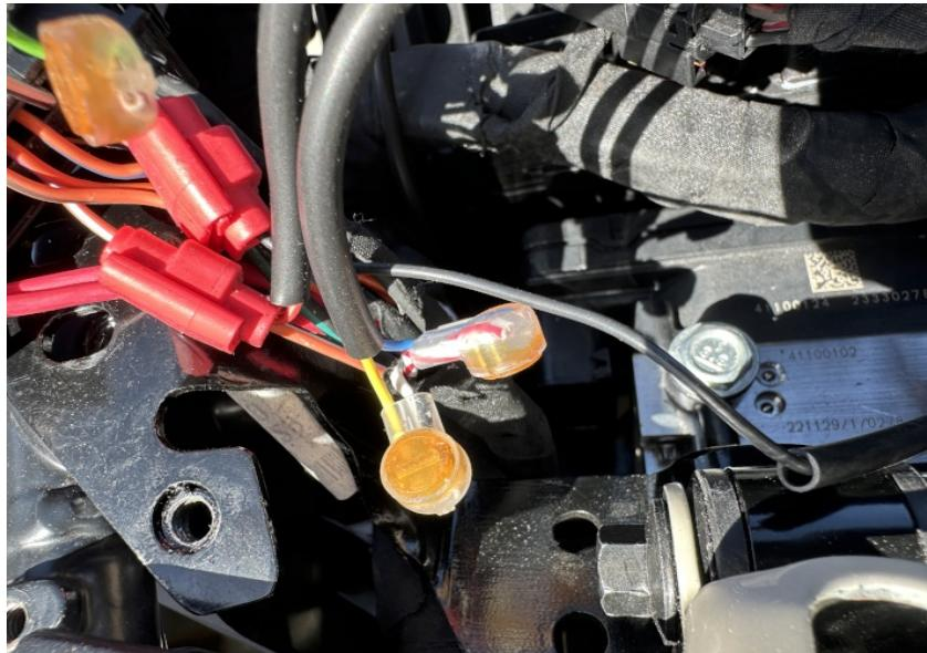
Splice the SH Red wire to the Orange/White wire of the ABS connector. Use a red wire tap connector.
