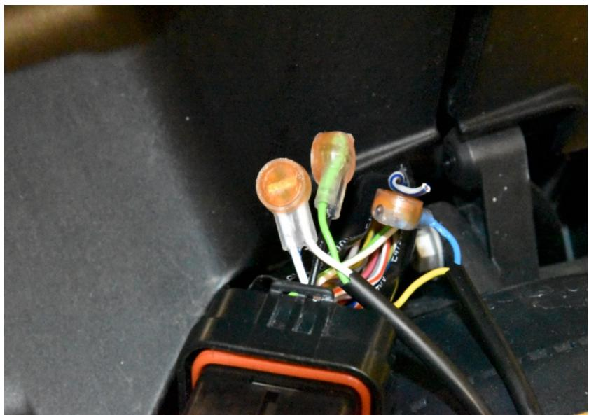
Connect the SH Yellow wire to the White/Blue wire end, which is at the wiring harness side. Use a yellow butt connector.
