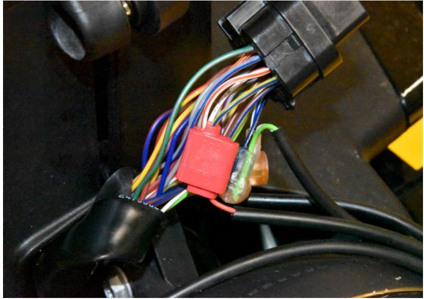
Splice the SH Black wire to the Brown/Blue wire of the dashboard connector. Use a red wire tap connector.
