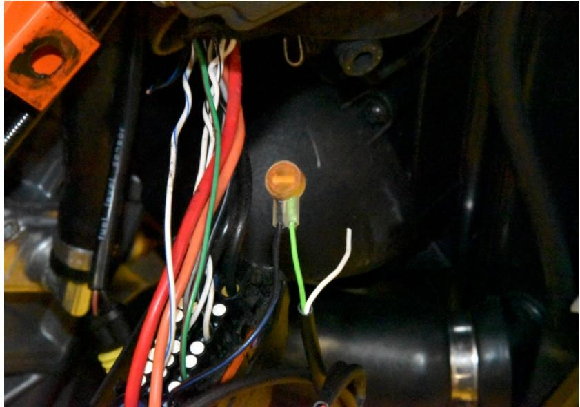
Connect the SH Blue wire to the Black/Blue wire end, which is at the wiring harness side. Use a yellow butt connector.
