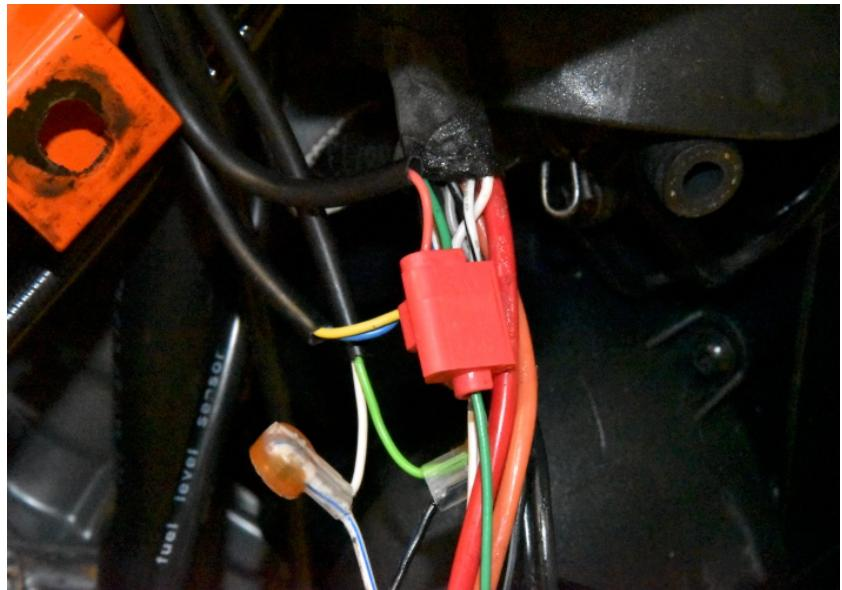
Splice the SH Black wire to the Brown wire of the right lamp connector. Use a red wire tap connector.
