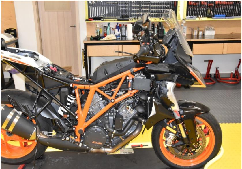
Locate the ABS connector on the right side.
