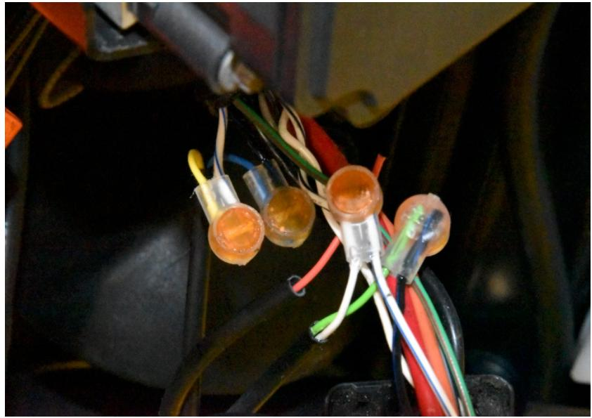
Splice the SH Red wire to the Green/Red wire of the ABS connector. Use a red wire tap connector.
