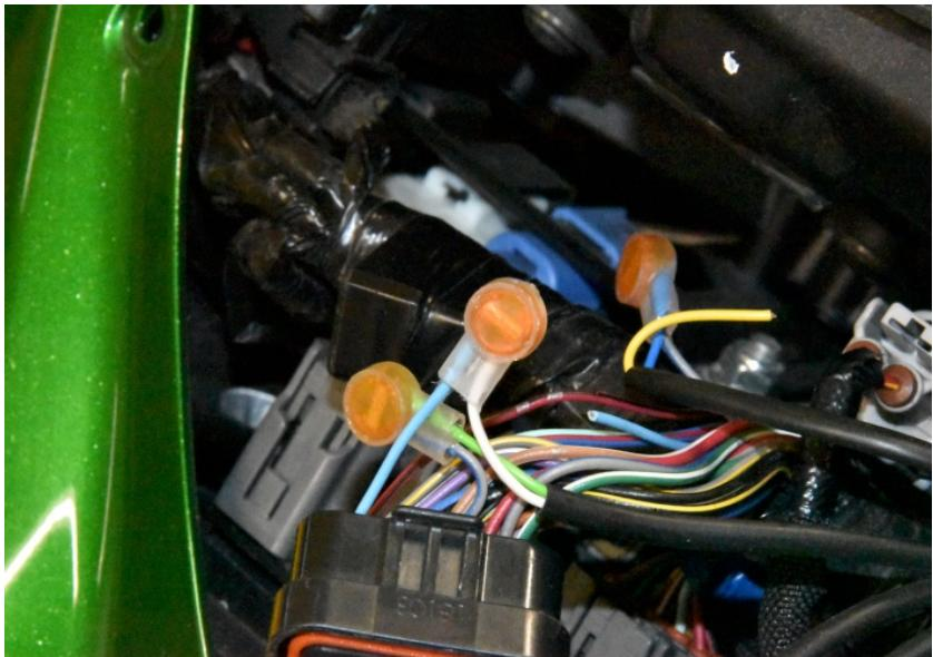
Connect the SH Yellow wire to the Light Blue wire end, which is at the wiring harness side. Use a yellow butt connector.
