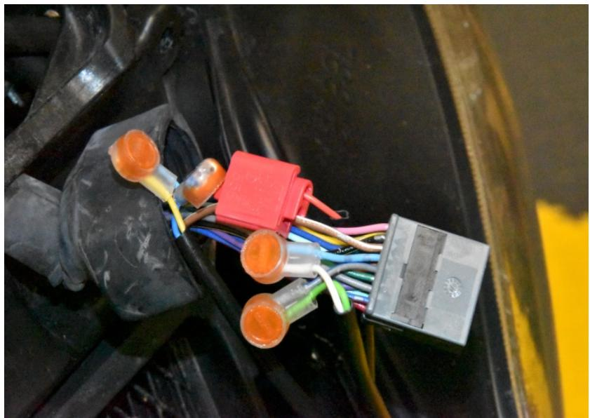
Splice the SH Black wire to the Black/Yellow wire of the dashboard connector. Use a red wire tap connector.
