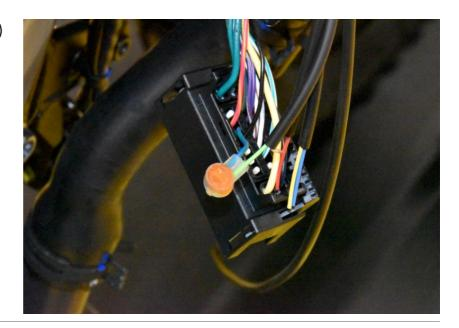
Connect the SH Blue wire to the Blue/Green wire end, which is at the wiring harness side. Use a yellow butt connector.
