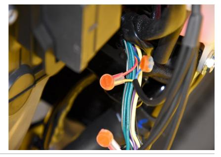
Splice the SH Red wire to the Black wire of the ABS connector. Use a red wire tap connector.
