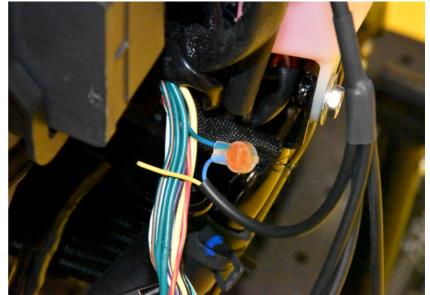
Cut the Red/Yellow wire about 2,5cm (1") of the connector.(Pin #12)
