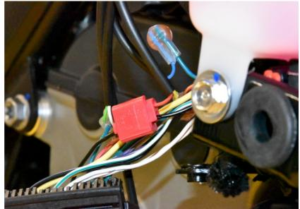
Splice the SH Black wire to the Green wire of the ABS connector. Use a red wire tap connector.
