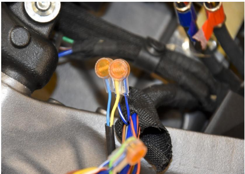
Splice the SH Red wire to the Orange/Blue wire of the ABS connector. Use a red wire tap connector.
