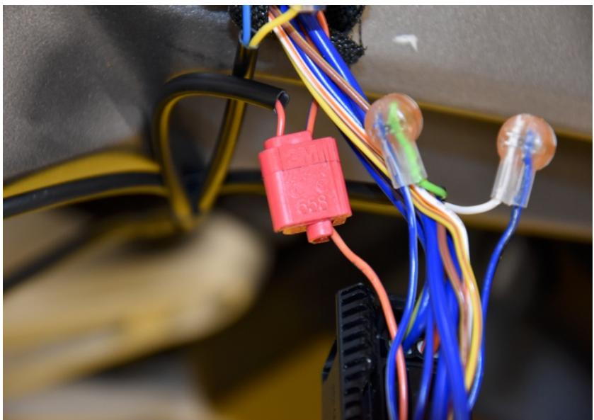
Splice the SH Black wire to the Blue wire of the diagnostic power connector. Use a red wire tap connector.
