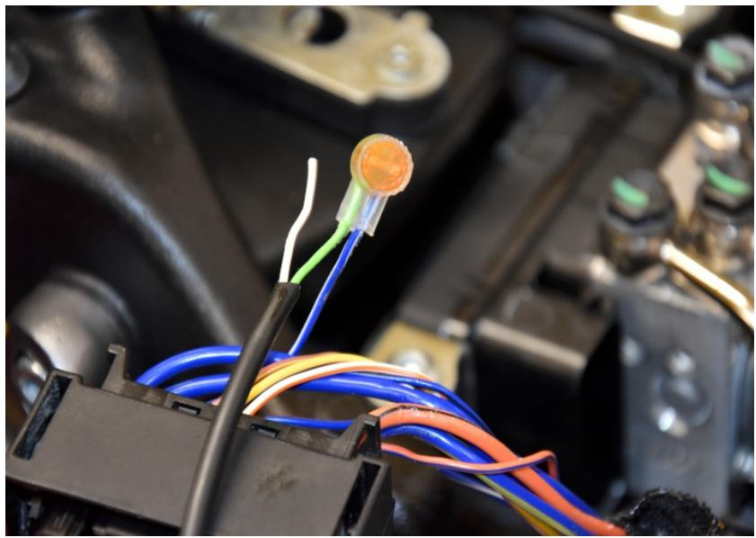
Connect the SH Blue wire to the Blue/White wire end, which is at the wiring harness side. Use a yellow butt connector.
