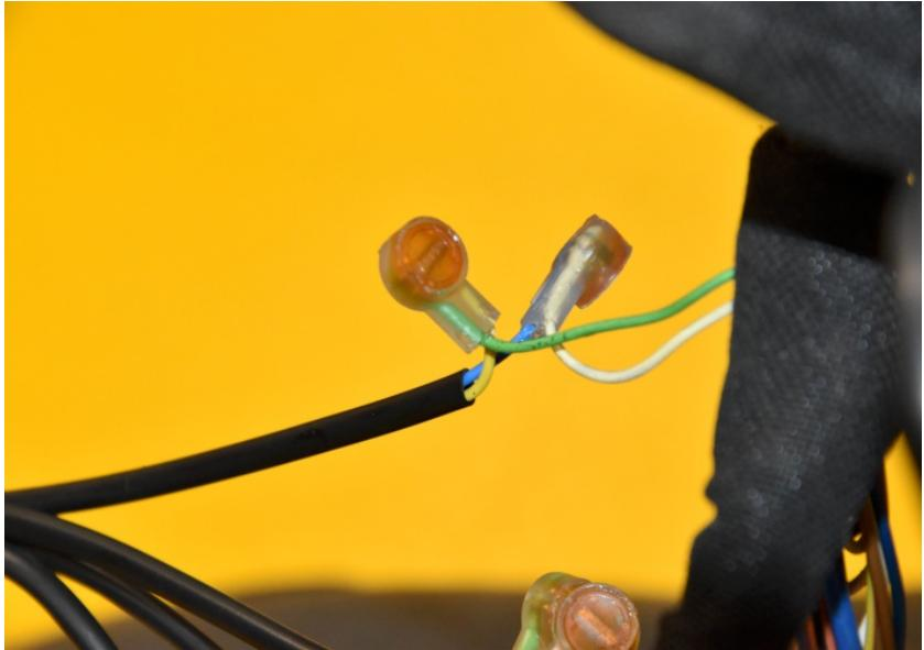
Splice the SH Red wire to the Orange/Blue wire of the ABS module. Use a red wire tap connector.
