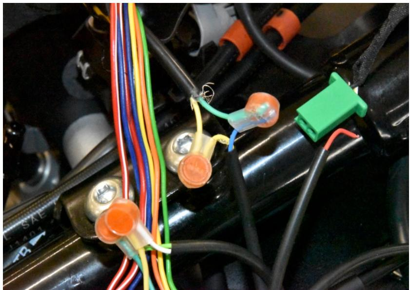
Splice the SH Red wire to the Blue wire of the ABS connector. Use a red wire tap connector.
