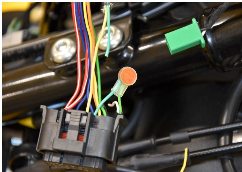
Connect the SH Blue wire to the Light Blue wire end, which is at the wiring harness side. Use a yellow butt connector.
