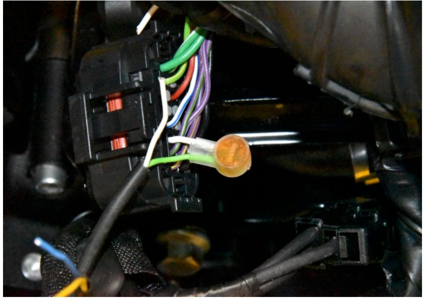
Connect the SH Blue wire to the White wire end, which is at the wiring harness side. Use a yellow butt connector.
