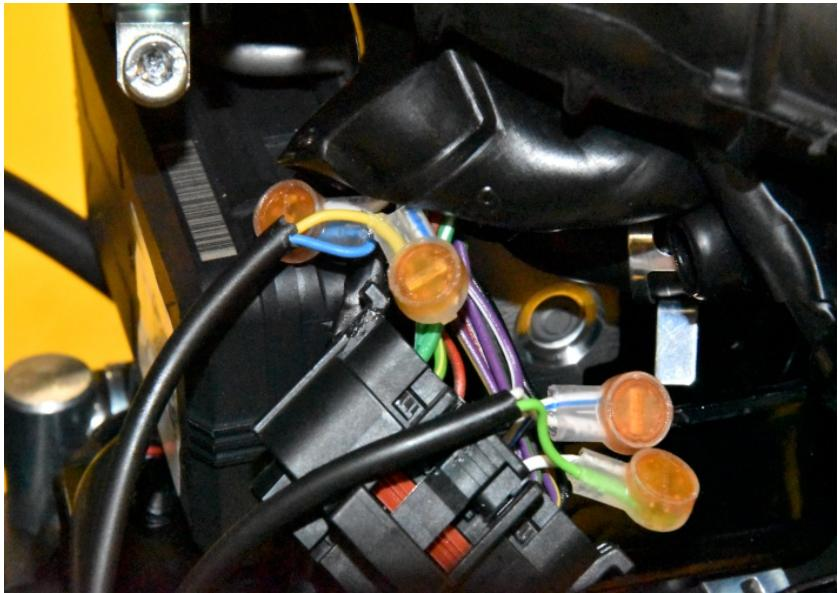
Splice the SH Red wire to the Red/Brown wire of the ABS connector. Use a red wire tap connector.
