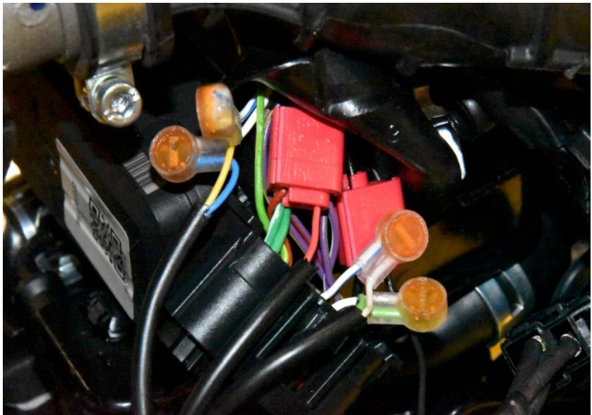
Splice the SH Black wire to the Black wire of the ABS connector. Use a red wire tap connector.
