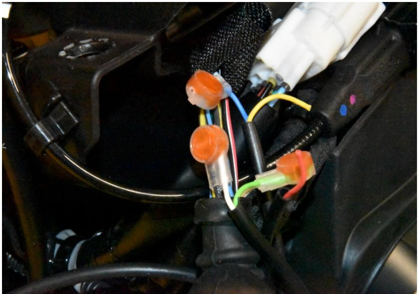
Connect the SH Yellow wire to the Black wire end, which is at the wiring harness side. Use a yellow butt connector.
