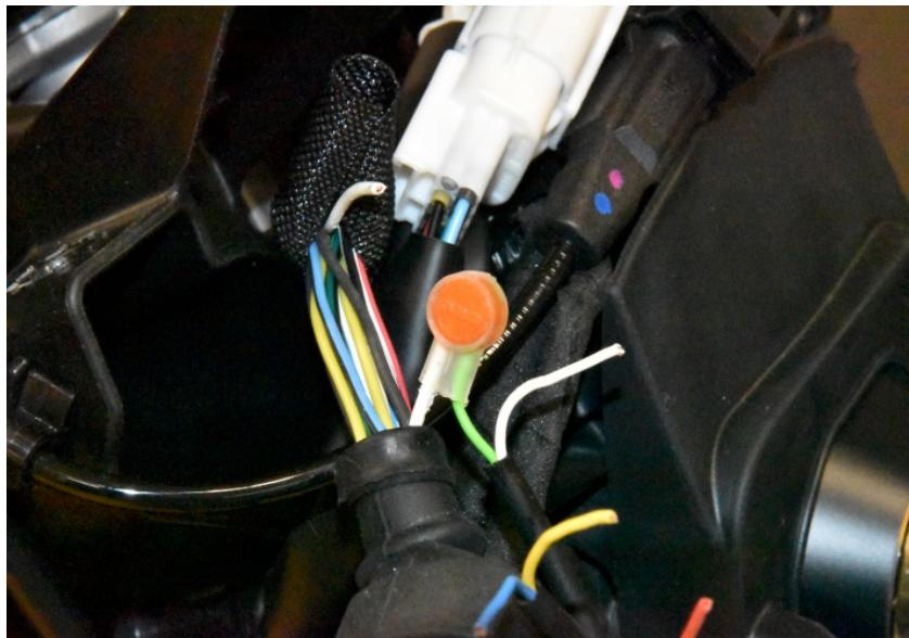
Connect the SH Green wire to the White wire end, which goes to the dashboard. Use a yellow butt connector.
