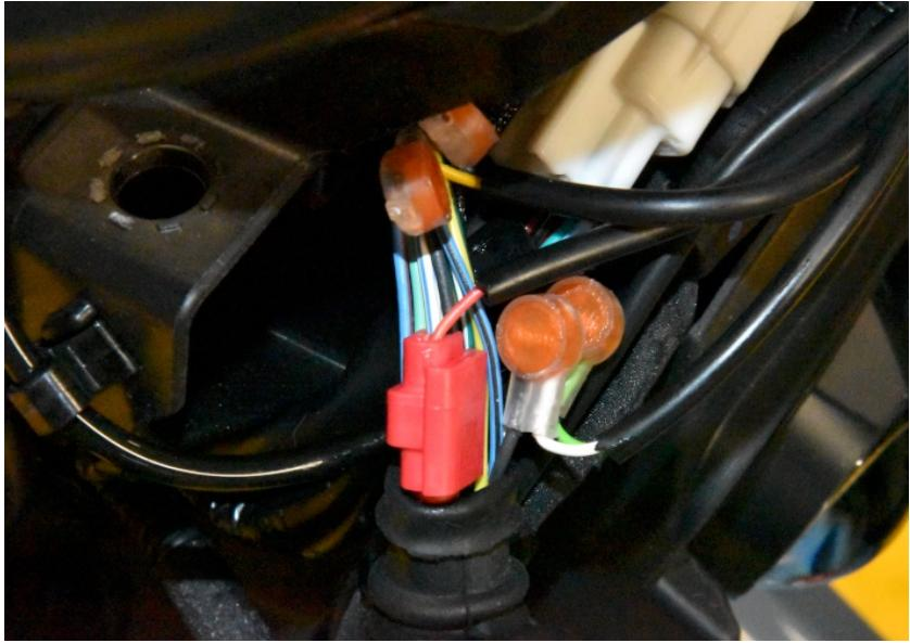
Splice the SH Black wire to the Black/White wire of the diagnostic connector. Use a red wire tap connector.
