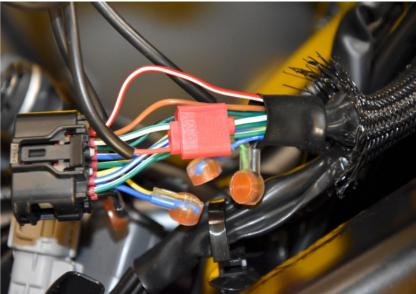
Splice the SH Black wire to the Black/White wire of the dashboard connector. Use a red wire tap connector.
