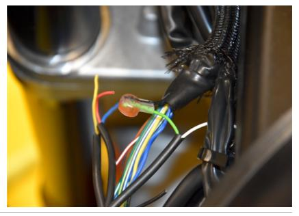
Connect the SH Blue wire to the Black wire end, which is at the wiring harness side. Use a yellow butt connector.
