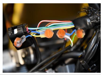
Splice the SH Red wire to the White/Green wire of the dashboard connector. Use a red wire tap connector.
