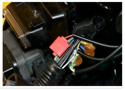
Splice the SH Black wire to the Black/White wire of the dashboard connector. Use a red wire tap connector.
