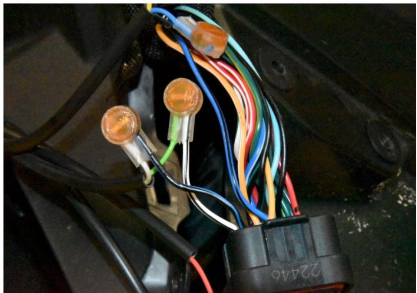
Connect the SH Yellow wire to the Black/Blue wire end, which is at the wiring harness side. Use a yellow butt connector.
