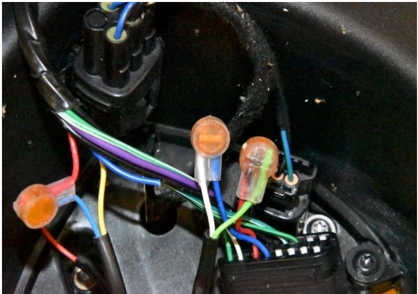
Connect the SH Yellow wire to the Blue wire end, which is at the wiring harness side. Use a yellow butt connector.
