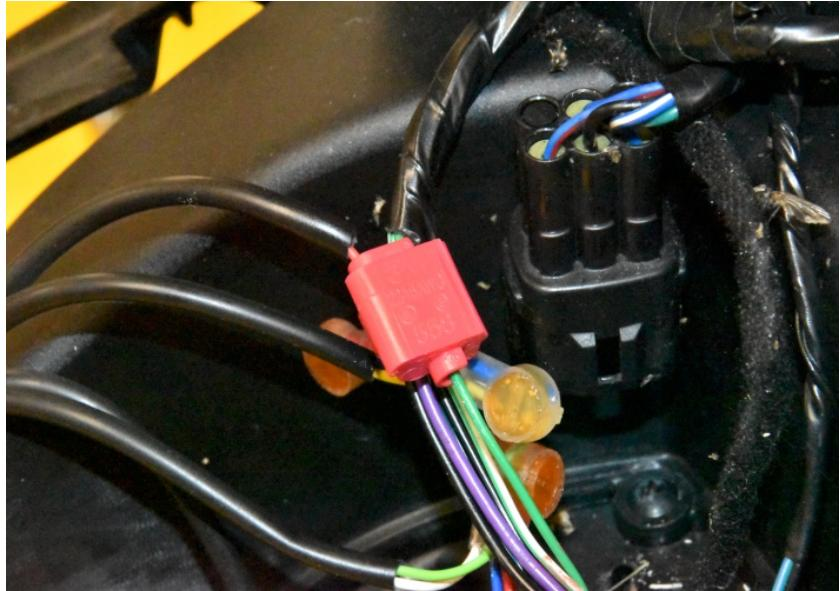
Splice the SH Black wire to the Black wire of the dashboard connector. Use a red wire tap connector.
