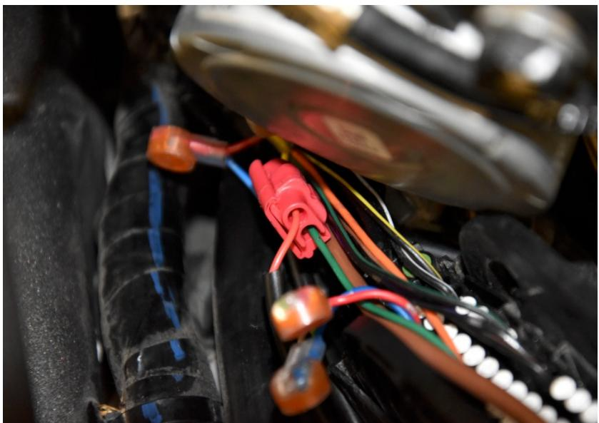
Splice the SH Black wire to the Black wire of the auxiliary power outlet connector. Use a red wire tap connector.
