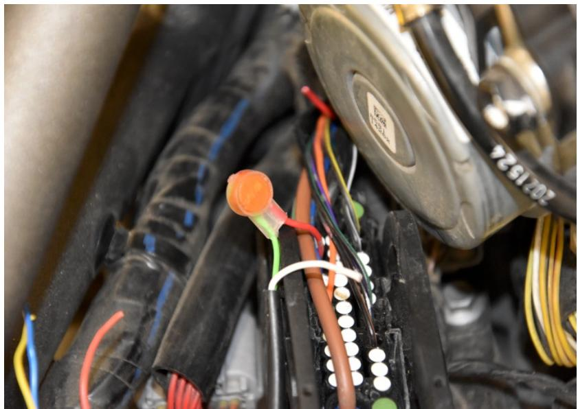
Connect the SH Blue wire to the Red wire end, which is at the wiring harness side. Use a yellow butt connector.
