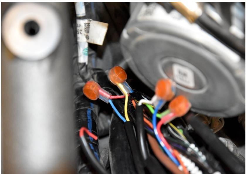
Splice the SH Red wire to the Green wire of the ABS connector. Use a red wire tap connector.
