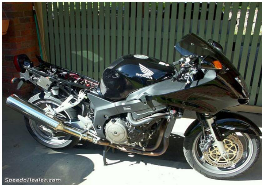
Lift up or remove the fuel tank.
