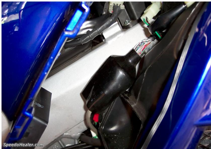
Locate the vehicle speed sensor connectors in a dust boot.
