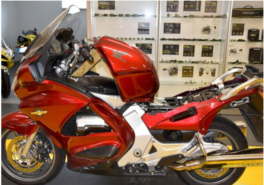
Locate the vehicle speed sensor connectors in a dust boot on the right side under the side fairing.
