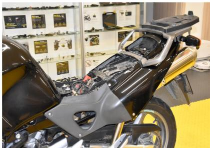
Locate the vehicle speed sensor connectors.
