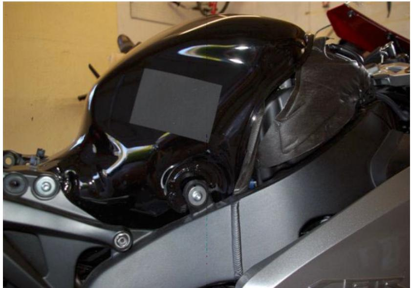
Lift up or remove the fuel tank.
