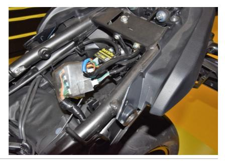
Locate the speed sensor connector.
