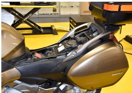
Locate the vehicle speed sensor connectors.
