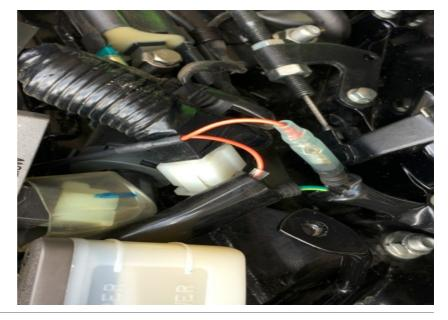
Wrap the wires and cables with black tape neatly.
