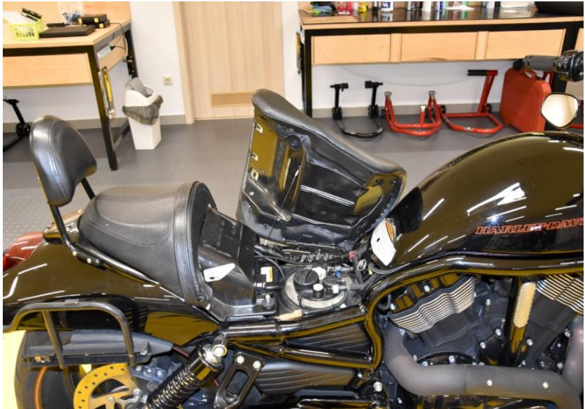
Locate the vehicle speed sensor connectors.
