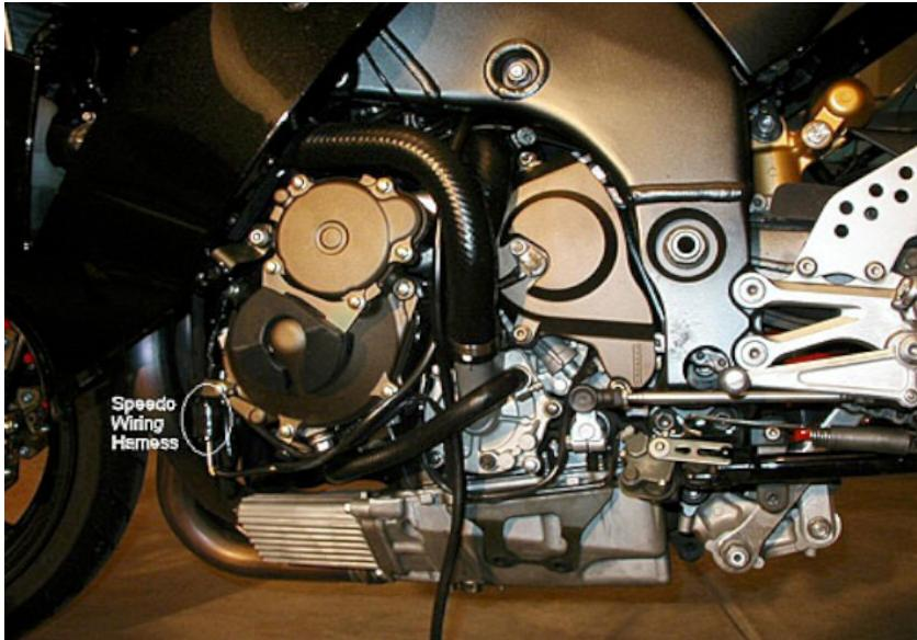
Locate the vehicle speed sensor connectors.
