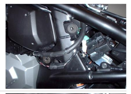
Plug the SpeedoHealer connectors in-line with the vehicle speed sensor connectors.
