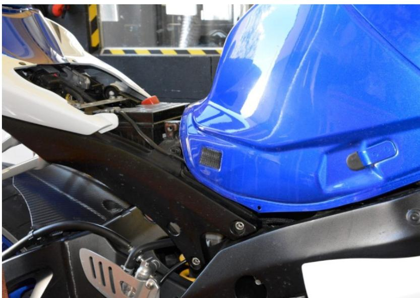
Lift up or remove the fuel tank.
