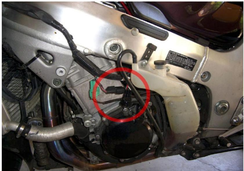
Locate the vehicle speed sensor connector.
