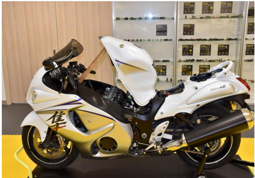
Lift up or remove the fuel tank.
