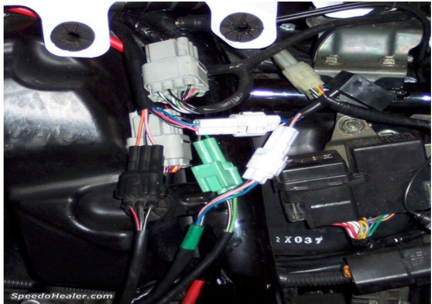
Locate the vehicle speed sensor connectors.
