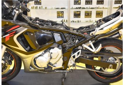
Locate the vehicle speed sensor connectors.
