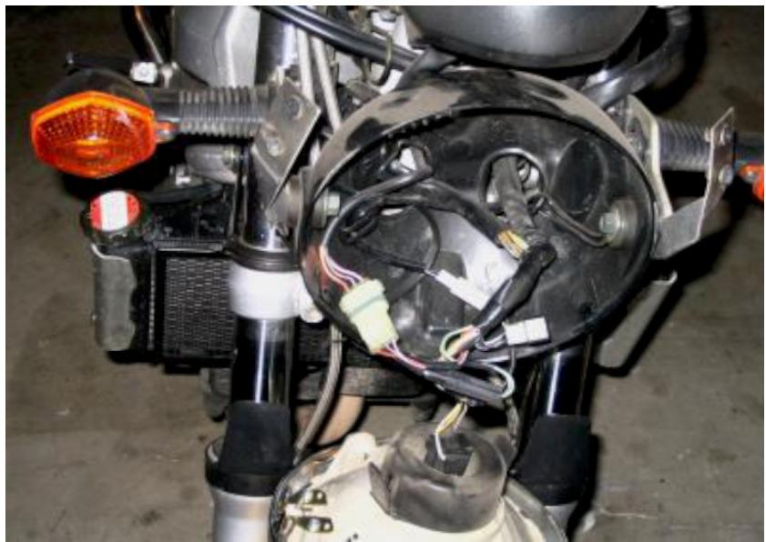
Locate the vehicle speed sensor connector.
