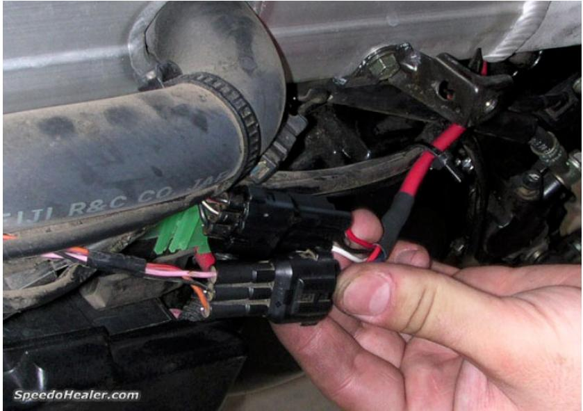
Locate the vehicle speed sensor connector.
