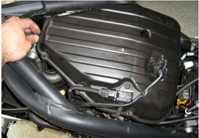
Locate the vehicle speed sensor connectors.
