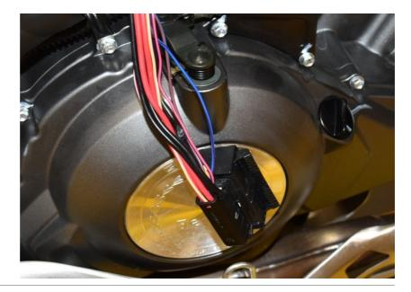
Connect the SpeedoHealer White wire to the Blue/Purple wire end, which is at the ABS connector side.
