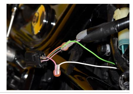
Splice the SpeedoHealer Red wire to the Brown wire of the fuel pump connector.
