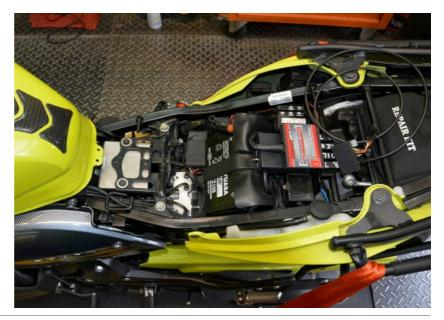
Remove the black frame cover at the left side below the fuel tank.
