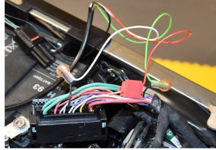
Splice the SpeedoHealer Red wire to the Orange wire of the ABS ECU connector.
