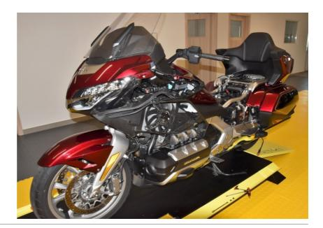
Remove the fairings around the fuel tank and locate the ECU.
