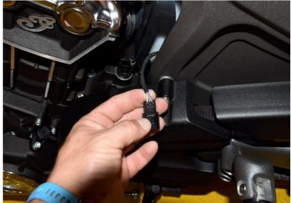
Cut the Green/Brown wire about 4cm (1.5") away from the speed sensor connector.
